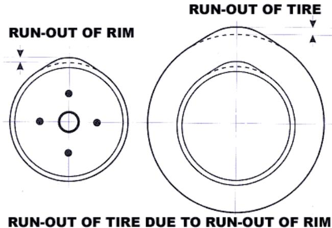
To resolve vibration problems, the run -out of tire and rim should be measured, then matched in the following manner:
